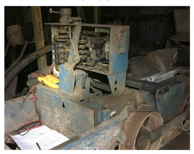
I have also included these shots of the original Sevcon Contactors, that are rarer than hens teeth, the second with the arc chutes removed.
